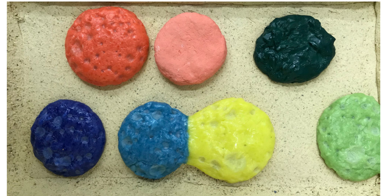
33. Clay samples based on parian mixed with stains, cellulose fiber and hydrated calcium borate.
