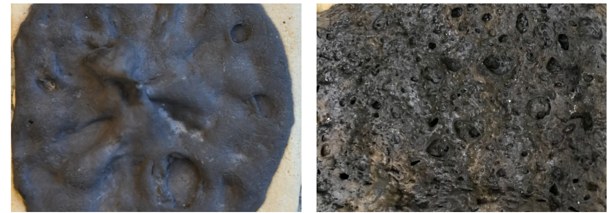
28. Two types of surfaces I developed for the project. Copper oxide prevails in the first clay, in the second one the component changing the colour and surface texture is cobalt oxide.
