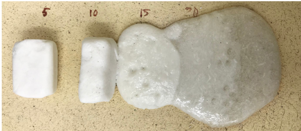
32. Clay samples based on parian mixed with hydrated calcium borate after high firing at 1200 C.
