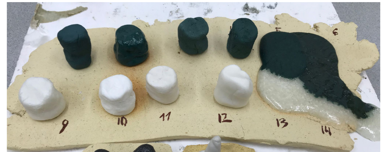
30. The parian and porcelain based mass mixed with (from left to right): frit A3383P, frit 2030, glaze WT 13000, NT 13000, gerstley borate and hydrated calcium borate in proportions of 75% to 25%.
