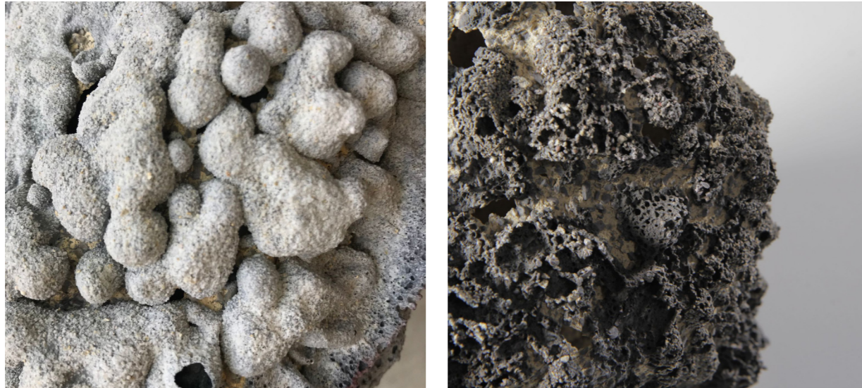
21. Test of black lava glaze fired submerged into containers with quartz sand 0,7-1,2mm particle size.
