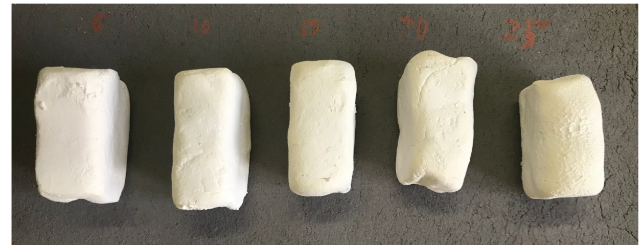
31. Clay samples based on parian mixed with hydrated calcium borate before firing.
