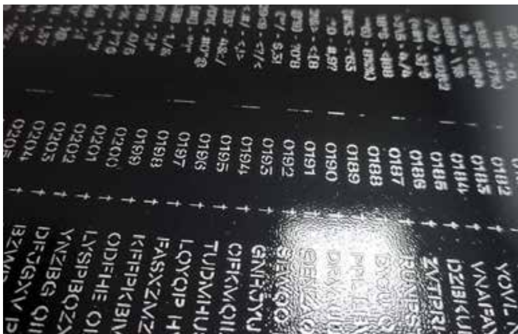
The resist layer, printed with black offset and siccatives
