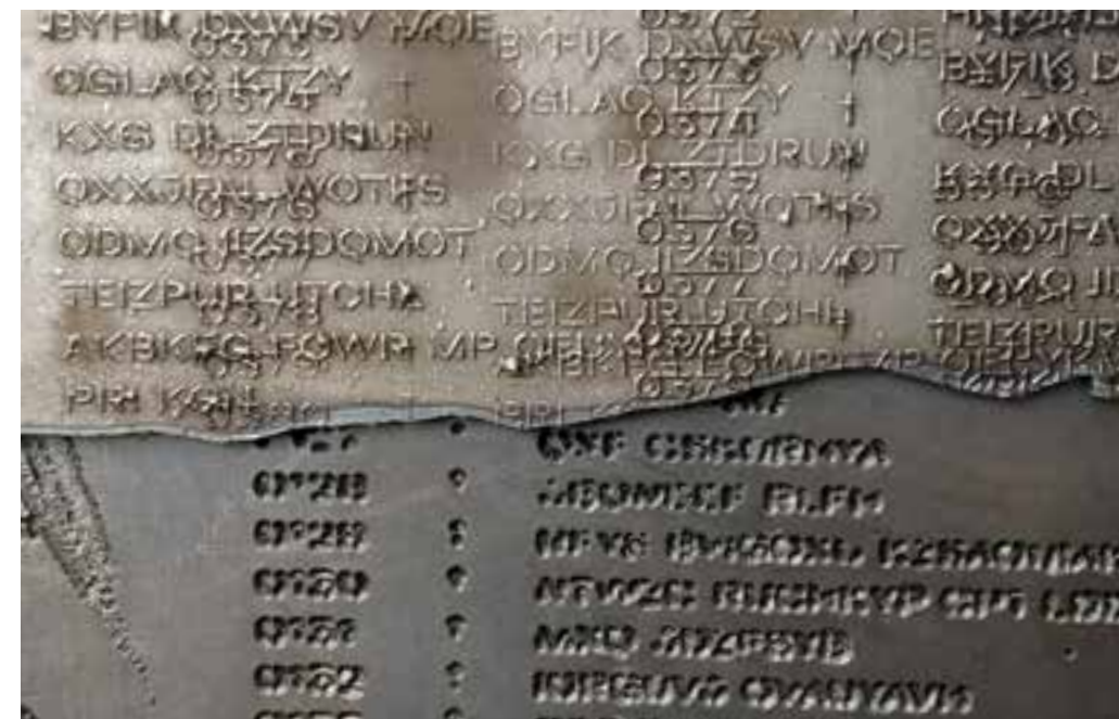
Top plate is etched with iron chloride. Bottom plate is etched with copper sulfate
