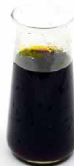
Edinburgh etch – Iron (III) Chloride and citric acid solution
