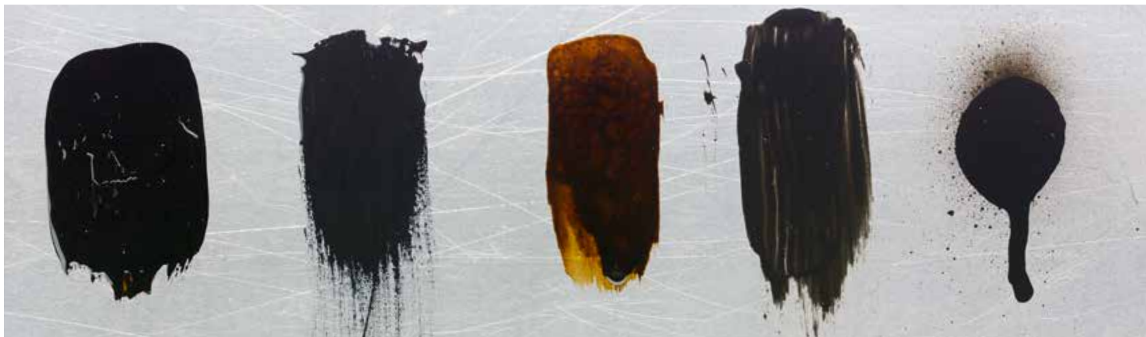
From left to right: tar, offset, varnish, solvent-based ink, acrylic spray on steel support
