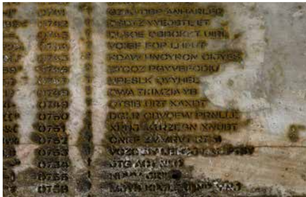
Plate etched with iron chloride. Resist used was solvent-based silkscreen ink
