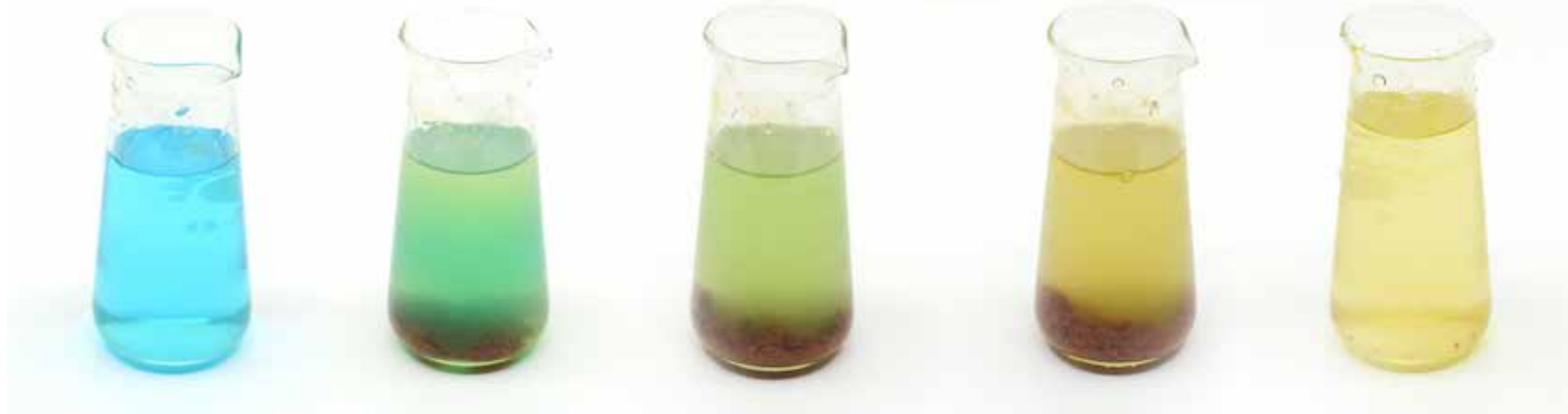
Different conditions of the copper sulfate solution. On the left a freshly mixed batch, on the right a spent solution
