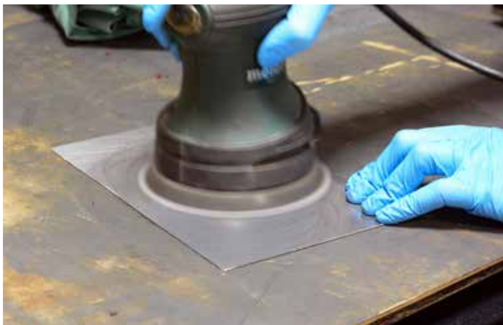
Sanding a plate with an orbital power sander
