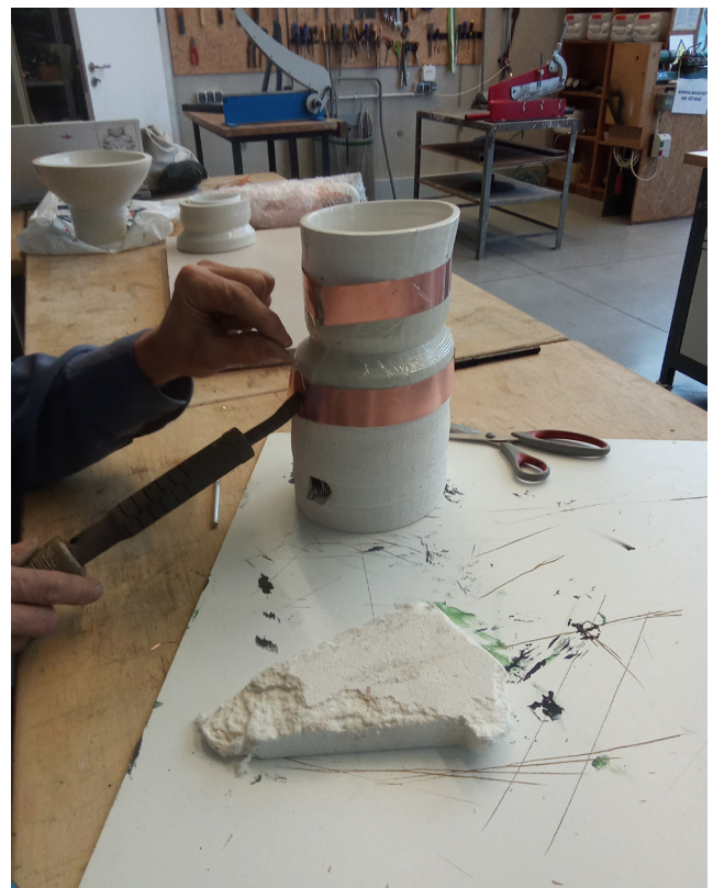
31. Adjusting the copper sheets
