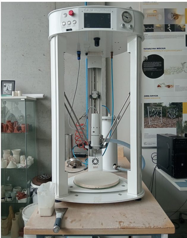
15. The ceramic 3D printer Gaia Multitool
