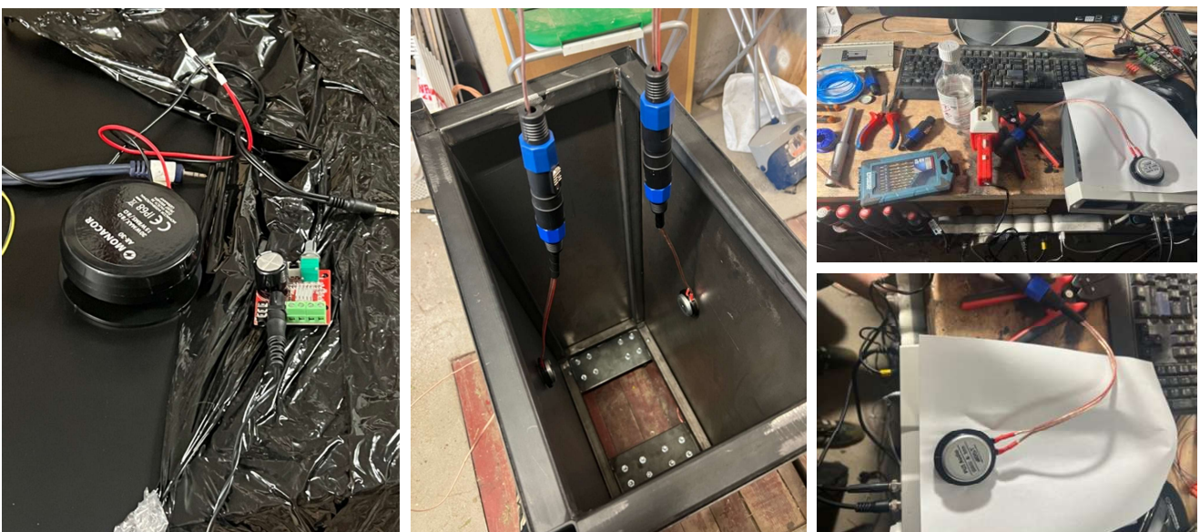
Figure 21 Placement of exciters (transducers) inside the steel structure. The units were mounted directly onto the inner panels and connected to an external amplifier, transforming the monolith into a resonant vibrational body.
