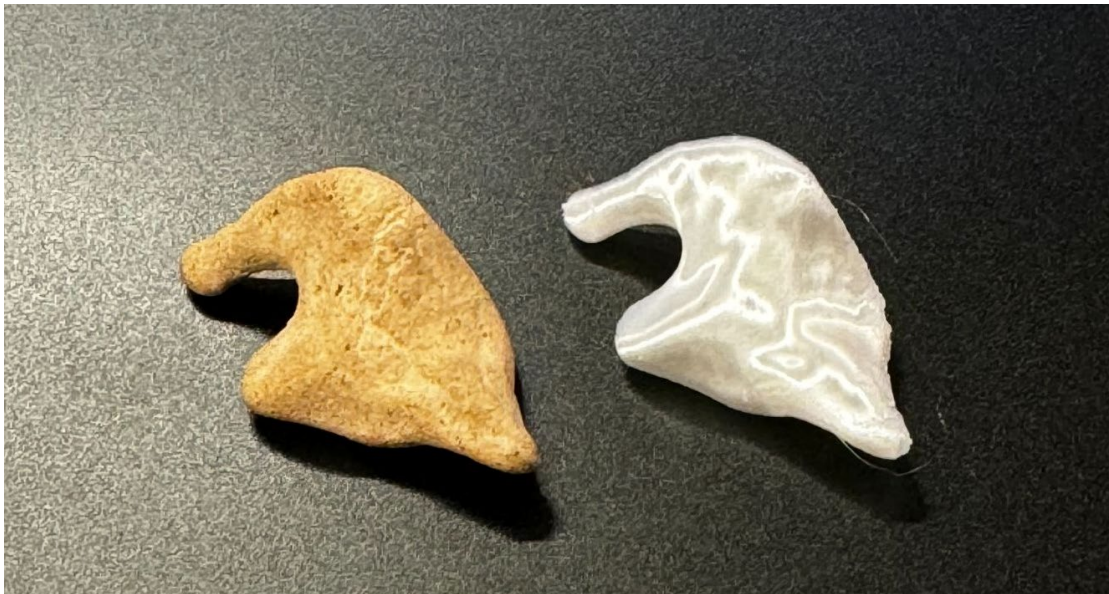
Figure 20. 3D print and the stone—a clearly visible change in form resulting from the use of a different material. Source: author's archive.
